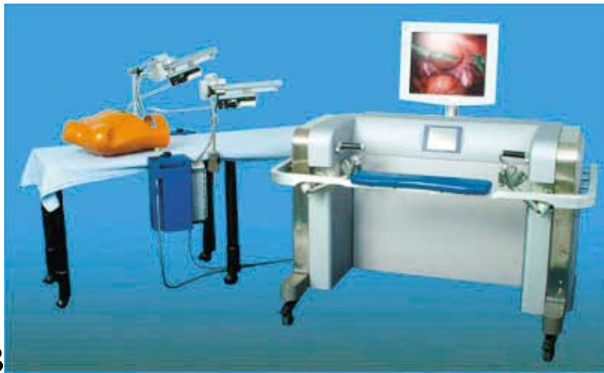
FIGURE 4. (a) Zeus and (b) Laprotek surgical robotic systems: lightweight, table-mounted, modular robotic arms (left) and surgeon consoles (right).
